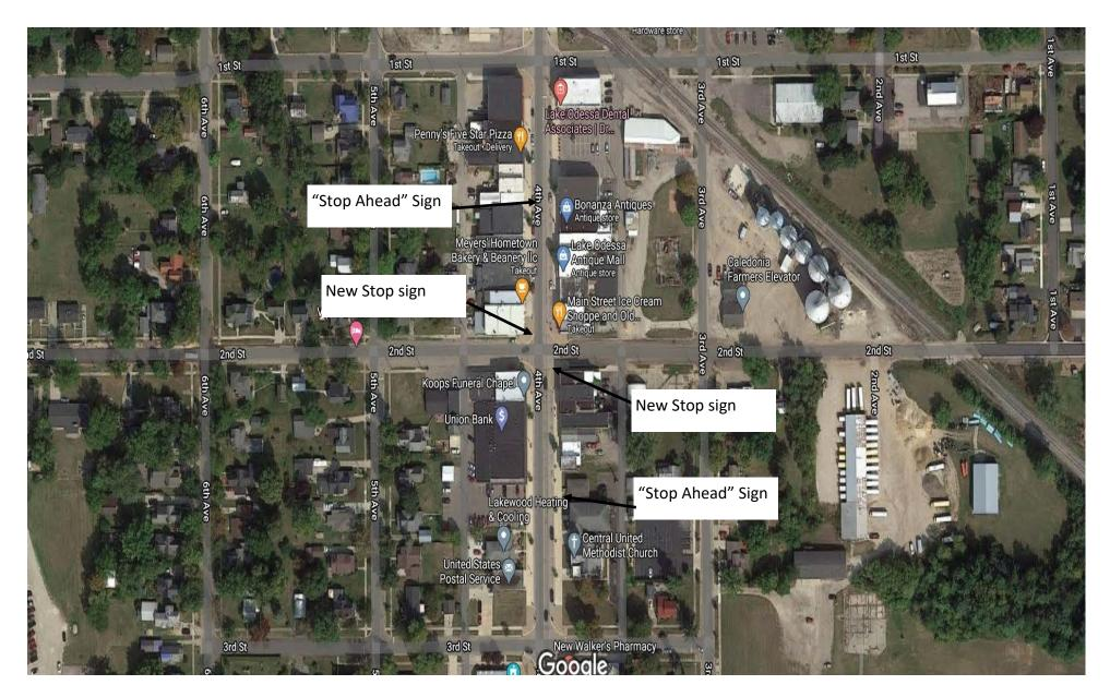
"Stop Ahead" signs will be placed on the street for maximum visibility, and will cause the need to close off one parking spot for each sign. "Stop" signs and "Stop Ahead" signs will be placed in concrete blocks and will not be installed into either the existing street or sidewalk. All will be temporary and able to be removed as needed and or at the end of the 90 days.
